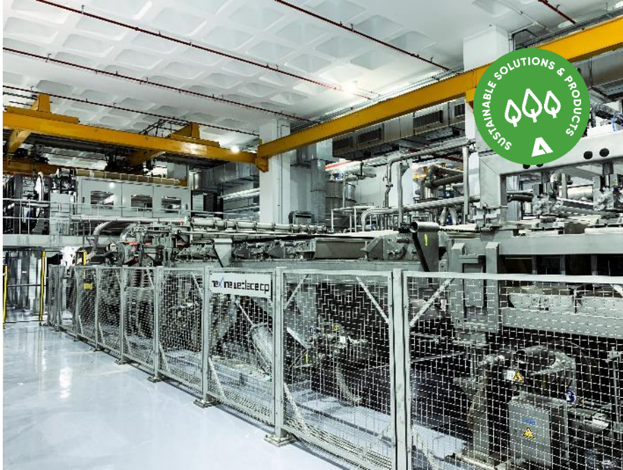
ANDRITZ neXline wetlace CP for the production of nonwoven roll goods for biodegradable wet wipes at Lotus Teknik Tekstil A.Ş., Türkiye
